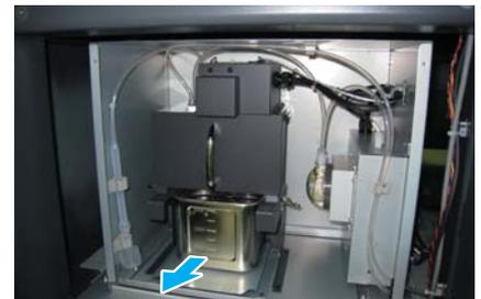
**8** Set the empty hot water tank into the water heating system and return the water heating system and the catch clip to the state of starting the operation.
