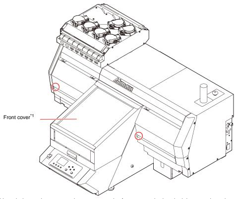
\*1: Although the carriage stops when you open the front cover, the interlock is not activated.
