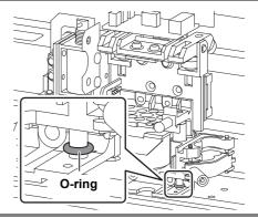
4 Attach the cutter guard while fitting the opening of the cutter guard to Z-shaped part of the yoke-bracket.
