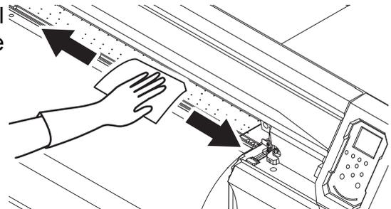
(6) Stick the NITOFロン® onto the platen.
