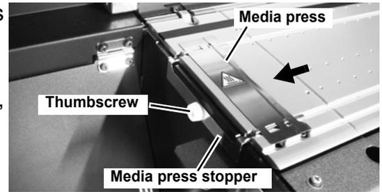
(5) Wet a Bemcot with the alcohol or diluted neutral cleansing agent, wring it out well, and use it to wipe the platen clean of grease.
