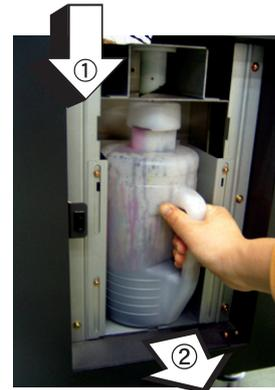
3. **Dump waste ink into a separate polyethylene tank.**
