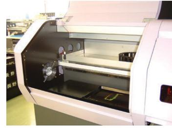
8. Wipe off the waste ink from the flushing tray with the paper towel containing washing liquid. Take the caked ink off by patting the tray.
