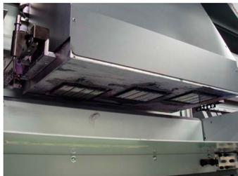
Clean the bottom surface of the slider and around the head with a cleaning stick.
