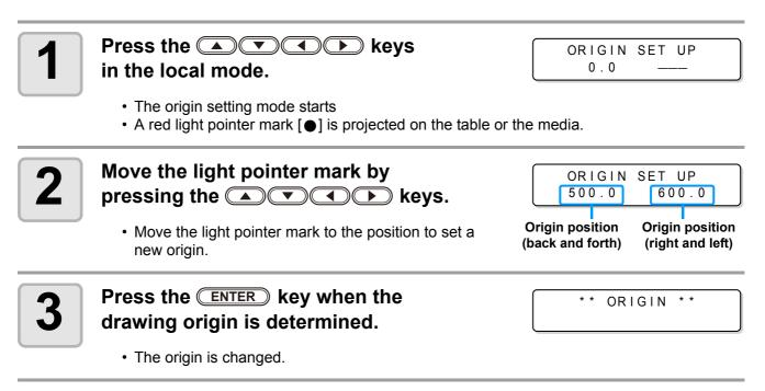
(mportant!) • The setting value for the origin set with the JOG keys is cleared by cutting the power.
