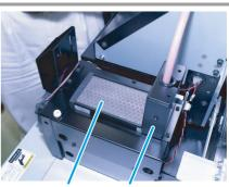
Mesh filter UV lamp connector cover
