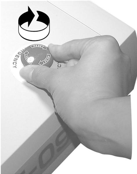
Turn the **EMERGENCY** button clockwise for unlocking.
