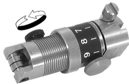
**Tighten the cutter stopper.**
